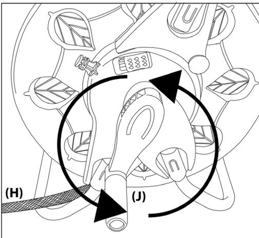
Rotate Reel handle (J) to wind in the hose pipe (H)
