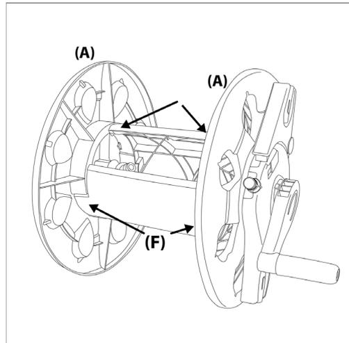
Connect Inner Reel (F) to both sides of the reel (A)
