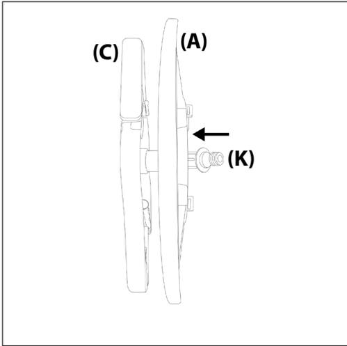
Connect angled connector set (K) through reel (A) & side panel (C)
