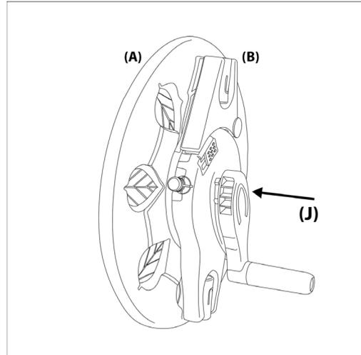
Connect reel handle (J) through side panel (B) and reel (A)
