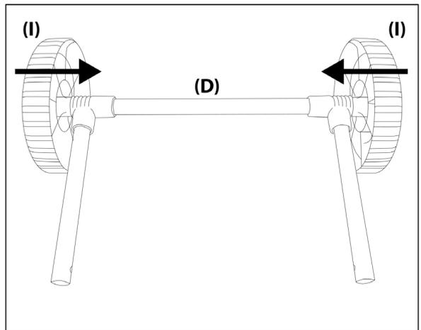
Connect wheels (I) to both sides of leg frame (D)
