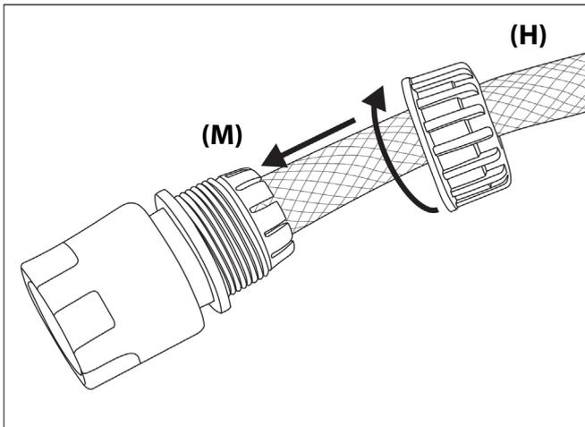
Insert end of Hose pipe (H) into Connector (M) and screw connector to lock hose in place
