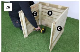
Now fix the remaining part C to part B again using 2x 60mm screws 1 at the top and 1 at the bottom approx.
