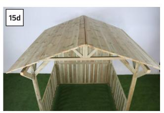
Interlock 9 x Roof Boards (I) and 1 x Square Edged Roof Board (H) and fix to Trusses E1 & E2 using 36 x 45mm Screws. (4 x Screws per board)
