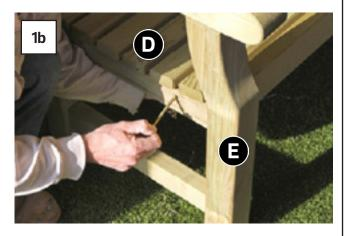
Locate Seat Assembly (A) into Side Assemblies (B) ensuring bolt-holes are aligned and insert 2no bolts per side (See Figs 1a & 1b). Locate washers and carefully thread nuts on to bolts, but do not tighten fully at this stage (hand tighten).
