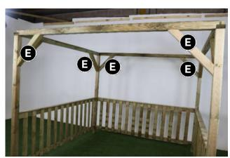
Fix 1 x Bracing (E) to Post (B) & Ring beam using 2 x 140mm Screws as shown above. Attach remaining Bracings (E) to Posts (B) & Ring beam using 14 x 140mm Screws, 2 x Screws per Bracing, 2 x Bracings per Post.
