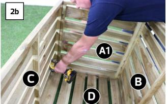
Fix Side Panel (A2) to Back Panel (B) using 2x 50mm screws placed evenly as per image.
