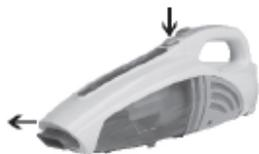
2. Press the release button to remove the dust container and pull the dust container away from the motor unit.
