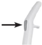
3. Press the On/Off switch on the handle to switch on the floor cleaner.
