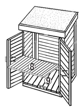
Step 6: Place the completed unit in position and adjust the Feet Part D to ensure that the unit is level and stable.
