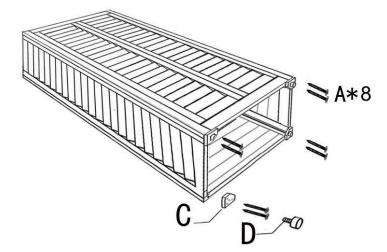
**Step 3: Secure the Feet Brackets** Part C to each corner of the unit using 8x Part A Long Screw.
