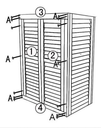
Step 2: Attach the Top Bar Part 3 and the Base Bar Part 4 to the frame by using 8x Part A Long Screw. Next fasten Parts 1 & 2 Left & Right Doors to the frame with 6xPart A Long Screw, ensuring that the slats are facing down.
