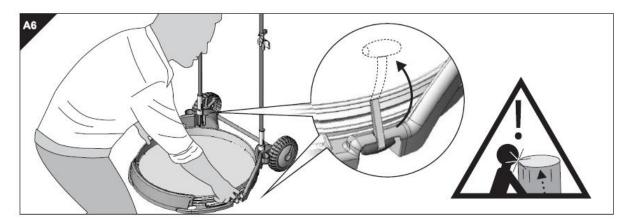
7. Expand the collection bag by unclipping the toggle on each side of the bag; be careful as this can expand quickly.
