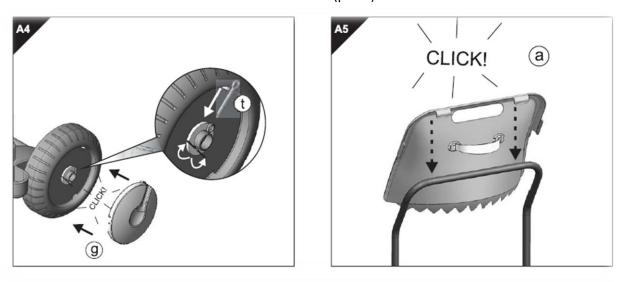
5. Bend the ends of the split pin around the axle, and then place the wheel hub (part g) into the wheel ensuring that this is clicked into place.
