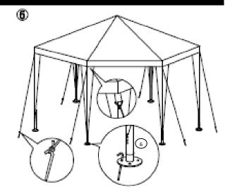
Fix ropes with stakes in top holes of each leg, and stake through one of the holes in the base plate into the ground.
