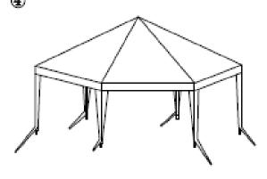
Pull cover tightly over the roof frame.
