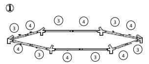
Lay out corner pieces and connect with frame (Parts 3 & 4).
