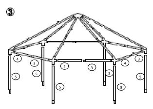
Connect parts nos. 5 with side corner joints.
