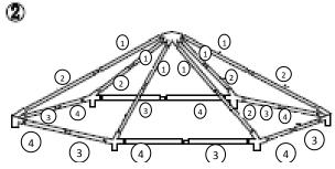
Connect tubes 1 & 2 between the centre connector and side corner joints.
