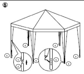
Connect parts nos. 6 with tubes nos 5 and push base plates into place.
