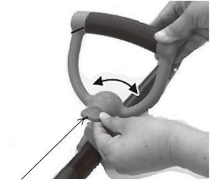
Undo screw to adjust handle to desired position.
