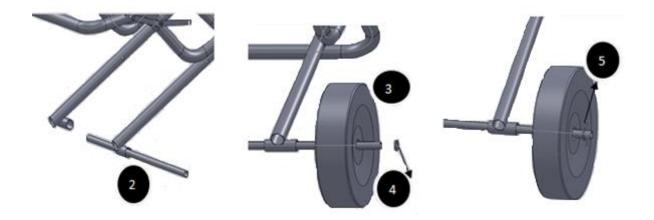
Step 2: Insert the Axle Part 2 into the frame. Attach the Wheels Part 3 into place followed by a Washer Part 4. Make sure the Wheels are fixed into place by using the Split Pin Part 5 through the hole in the Axle.
