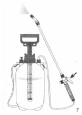
7. The sprayer will work when the trigger on the nozzle handle is pressed. To spray continuously, slide the trigger forward into lock position after pressing.
