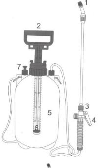
1. Attach the nozzle by screwing it on in a clockwise direction.
