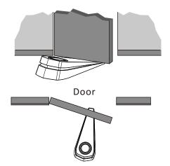
When the door opens, the alarm will be triggered
