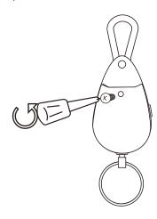
Unscrew the screw and remove the battery cover.
