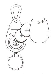
Put two CR2032 batteries (included) into the battery compartment with the positive side up
