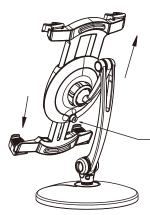
Pull along the arrow direction to adjust the appropriate distance
