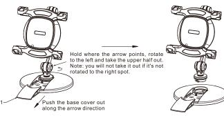
Push the base cover out along the arrow direction.
