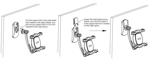
Insert the wall plate cover which is seperated in step 3. (note: you will not insert it if the upper half isn't rotated to the right spot)
