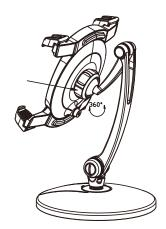
1. Rotate where the arrow points to the right to increase the torsion of the main body
