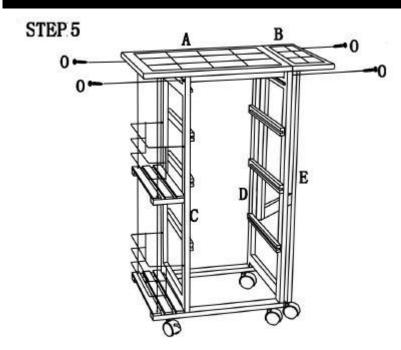
Attach top (assembled in step 2, part A & B) using screws O in positions as shown.
