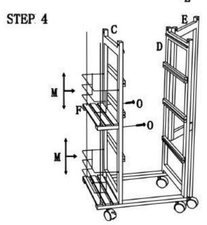
Turn over assembled parts and attach part F to part C with 2x screw O as indicated, then slide in part M 2x as shown.
