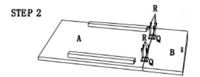
Connect part A with part B using screws R and brackets Q.
