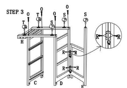
Connect part C and D via part H affixing screws R in the 4 positions indicated. Attach wheels S and T as shown in diagram and one wheel S on part E as indicated. Attach part E to part D using screws R and brackets Q.
