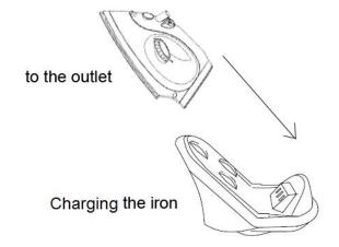
To charge the iron, place the iron on the power base.
