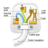
The diagram shows the key features of a correctly wired three-pin mains plug.
