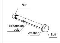
(Note: the nut and washer might be separated from the bolt during the process of transportation, please put them back into their original positions before you hammer them into the wall during installation.)
