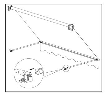
To retract the awning, wind the fabric to the closed position.
