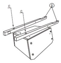
**Step 4** Slot in assembled wheel as shown.
